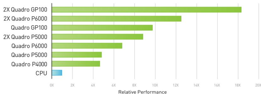
Tests run on a workstation with Intel Xeon E5-2697 V3, 14 cores 2.6GHz, 32GB RAM, running Win 7 64-bit SP1 and driver version 375.86. Performance testing completed with internal NVIDIA Iray tests at HD resolution.
