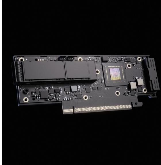
The NVIDIA® ConnectX®-9 SuperNIC™ supercharges gigascale AI computing workloads with support for per-port speeds of 800 gigabits per second (Gb/s) over InfiniBand and Ethernet. It delivers extremely fast, efficient network connectivity that significantly enhances system performance for AI factories and cloud platforms.
