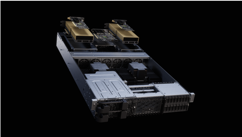
RTX PRO Server: 2U System Configuration 2x RTX PRO 6000 Blackwell Server Edition
