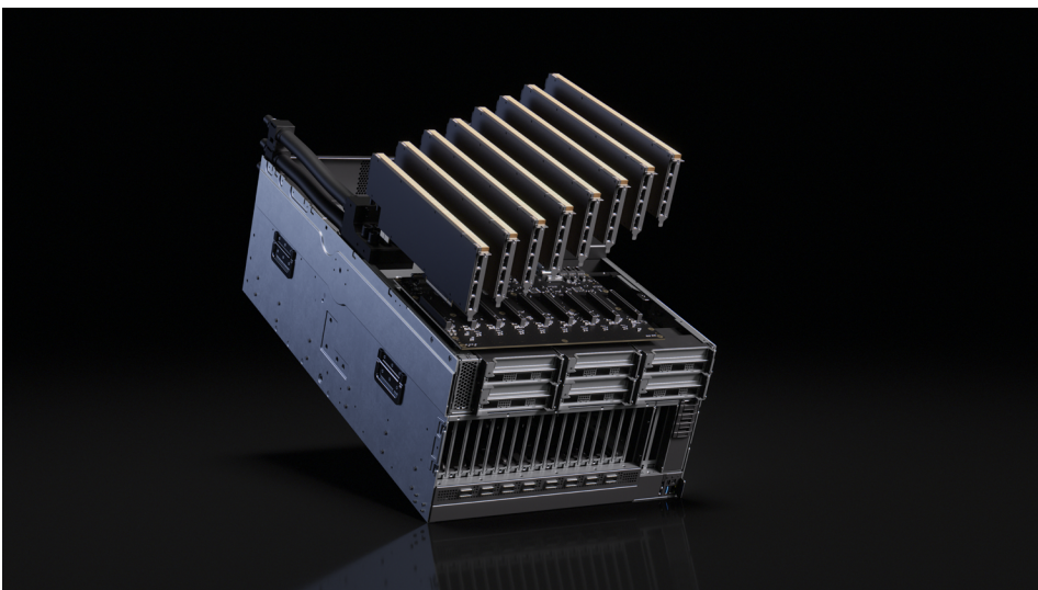
Liquid-Cooled RTX PRO Server: 6U System Configuration Up to 8x Liquid-Cooled RTX PRO 6000 Blackwell Server Edition
