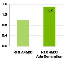
Tests run on an Intel Core i9-12900K Processor @ 3.2GHz (5.2GHz Turbo), 64GB RAM, Windows 11 Enterprise x64, MLPerf v2.1, NVIDIA Driver 525.89. Relative speedup for BERT Inference, INT8 precision. Performance based on pre-released build, subject to change.
