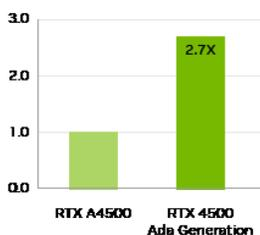
Tests run on an Intel Core i9-12900K Processor @ 3.2GHz (5.2GHz Turbo), 64GB RAM, Windows 11 Enterprise x64, NVIDIA Driver 525.49. CAD application performance based on internal testing of NVIDIA Omniverse Create with several models of varying size and render complexity. Performance is measured as frames rendered per second. NVIDIA DLSS 3 is enabled for NVIDIA RTX 4500 Ada Generation GPUs, DLSS 2 enabled for non-Ada generation GPUs. Performance based on pre-released build, subject to change.
