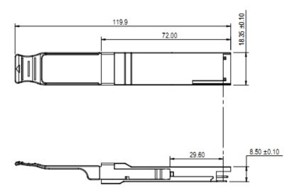
**Note:** External physical characteristics are subject to variation. This may include, but is not limited to, external case designs, pull tab colors and/or shapes, removal latch styles or colors, and label sizes and placement. These variations do not affect the function or characteristics of the transceivers.
